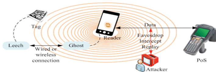
Fig. 2. Attack vulnerabilities on NFC payment systems.
