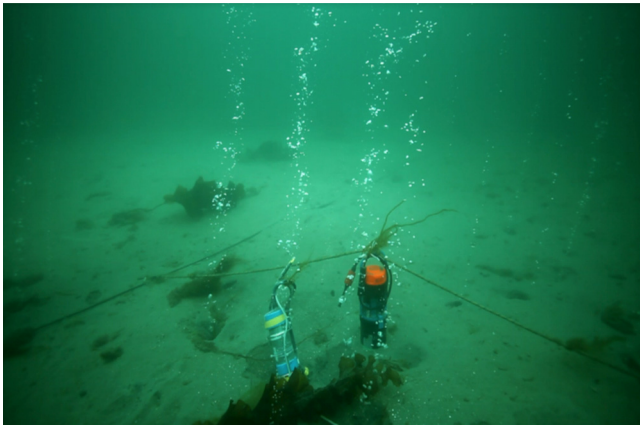
Fig. 10. In situ image of the release zone, showing bubble streams of CO 2 gas leaving the sea bed, pock marks can be seen at the base of the bubble streams caused by mechanical disturbance to the sediment. Photograph also shows various sensors deployed for monitoring, to the right is an Aanderaa Seaguard current meter equipped with a pCO 2 optode and a CTD to the left. The cable running across the seafloor is an Online pCO 2 /pH ISFET electrode sensor. The results from these sensors is discussed in detail in Atamanchuk et al. (2014).
