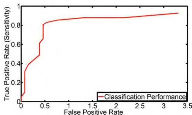
**FIGURE 12.** The receiver operating characteristic curve for the support vector machine classifier.
