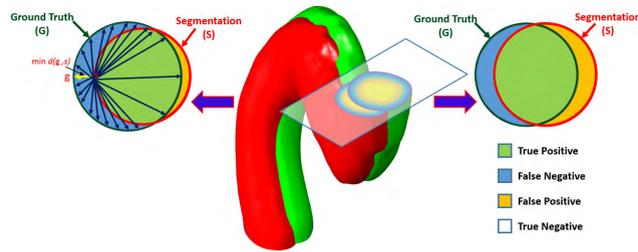
**FIGURE 3.** Illustration of the Dice coefficient, (right), and the Hausdorff evaluation, (left), metrics. Evaluation is performed in 3D while a 2D cross section is depicted for visualization simplicity.
