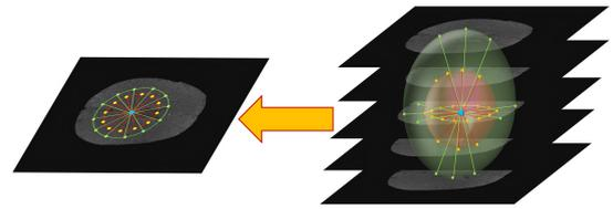
**FIGURE 2.** A 2D and 3D illustration of the proposed rotational and translational invariant neighborhood system. The center voxel and the neighborhood system are colored in blue and yellow respectively.
