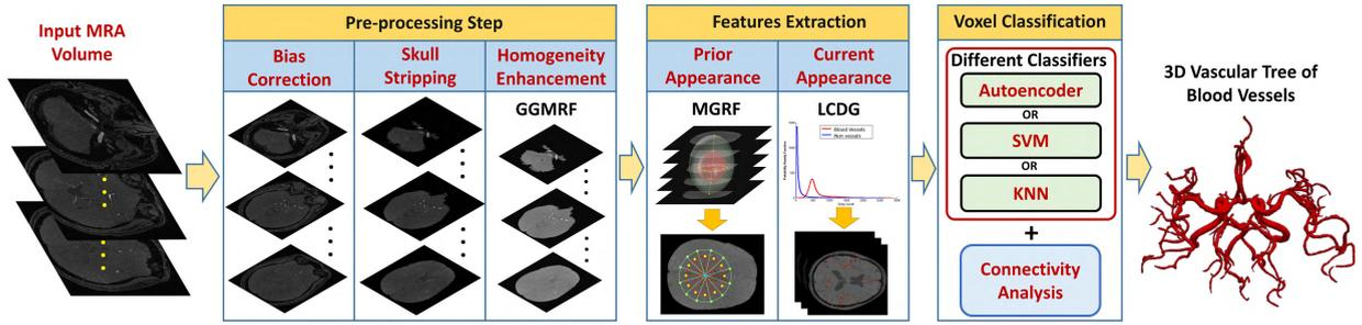
**FIGURE 1.** The proposed segmentation framework showing the step by step details starting from Pre-processing, feature extraction, voxel classification, and finally the post-processing.
