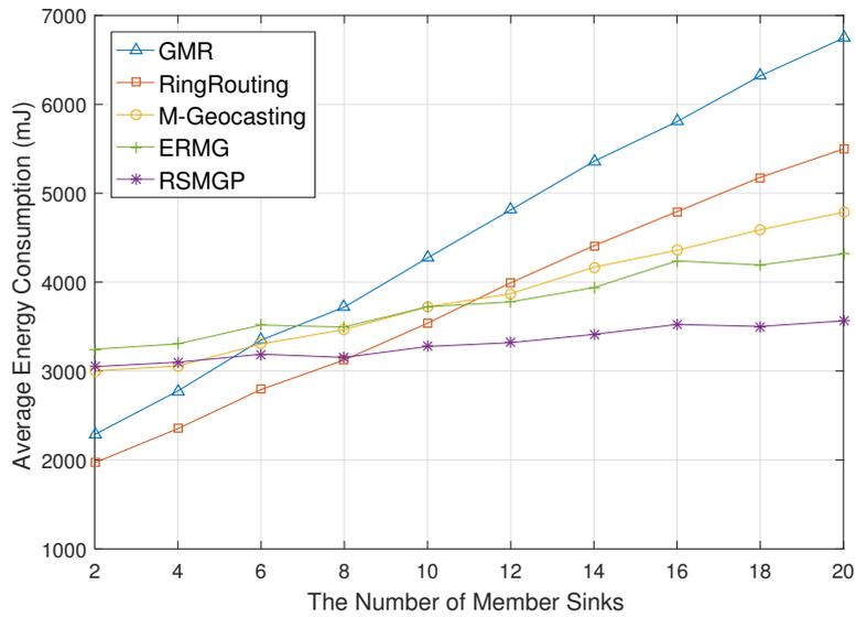
Figure 7. Energy consumption impacted by the number of member sinks.
