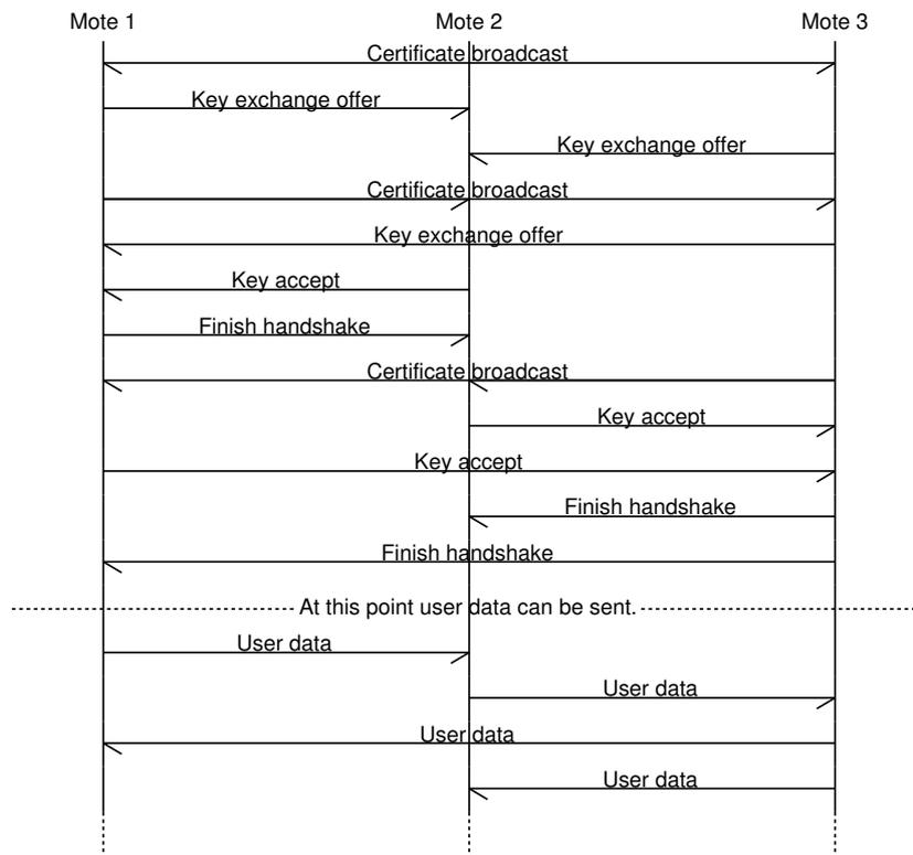
**Figure 1.** Example handshakes between three motes.
