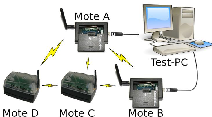
**Figure 4.** Configuration of the four-mote test bed.
