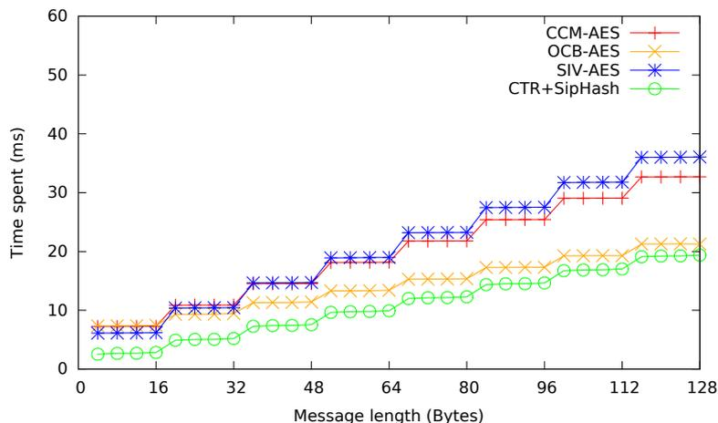
**Figure 8.** Time required for authenticated encryption with different modes. CCM, counter with cipher block chaining (CBC)-MAC.
