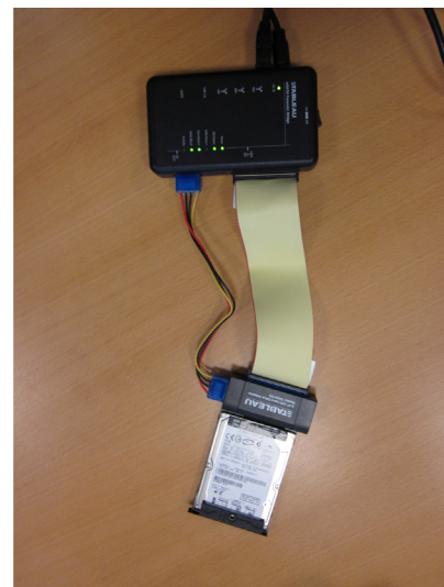
Fig. 2. The suspect hard disk connected (via IDE adapter) to the write blocker.
