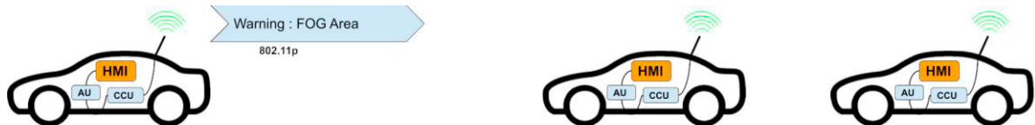
Fig.1: V2V communication based on the IEEE 802.11p
