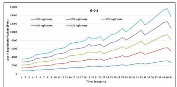
FIGURE 20. Loss in legitimate packets for  $TTD(t + 1)$  adjustment using algorithm 3 when  $\delta$  values vary between 0.5-0.9.
