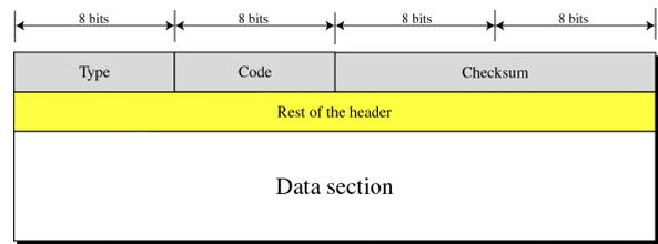
FIGURE 6. The fields of an ICMP packet.
