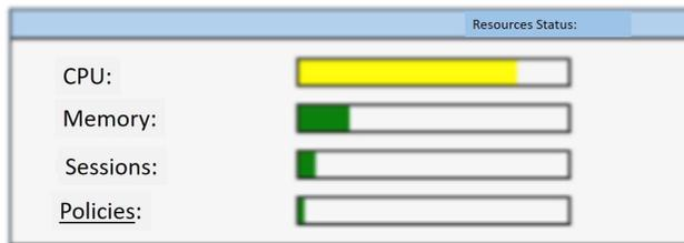
FIGURE 11. The effect of the BlackNurse attack on Juniper SSG 20 CPU performance.
