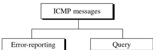
FIGURE 5. ICMP packet's types.
