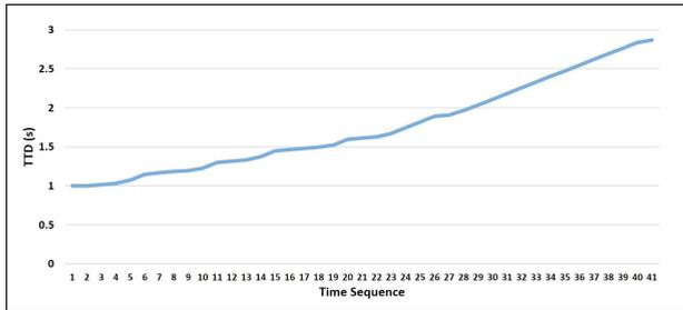
FIGURE 13.  $TTD(t)$  can increase indefinitely if attacker keeps increasing the attack rate,  $R_{max}(t)$ .
