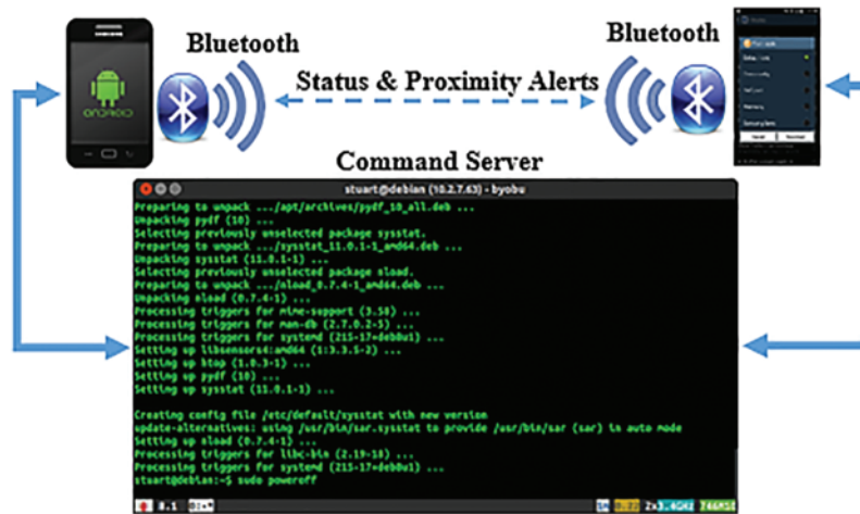
Figure 3: Bluetooth and command server communication
