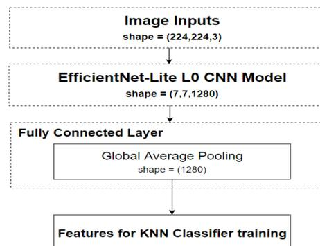
**FIGURE 16. CNN Model with Weights Frozen to Generate KNN Training Input.**
