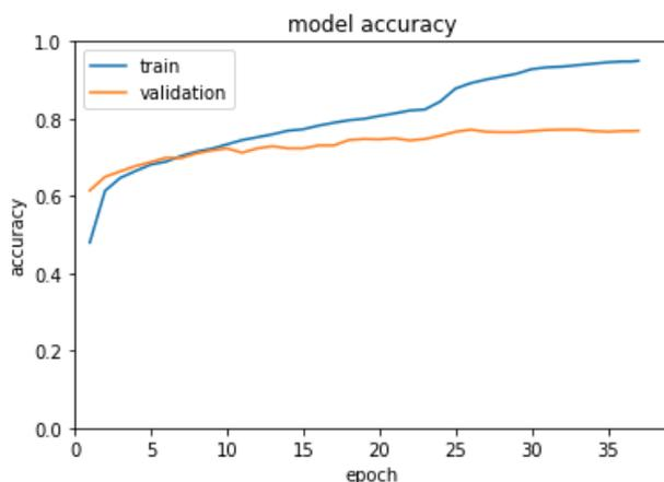
**FIGURE 12.** Model Training and Validation Accuracy vs Epoch for 0.001 Learning Rate.
