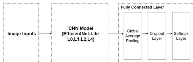
**FIGURE 6.** Network for EfficientNet-Lite Model Experiment.
