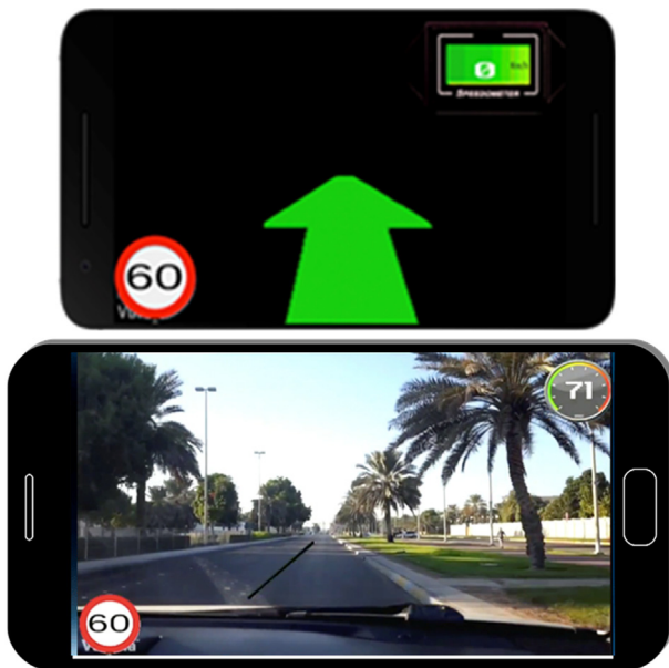
Fig. 8 Drive mode screens (lane detection and speed monitor).
