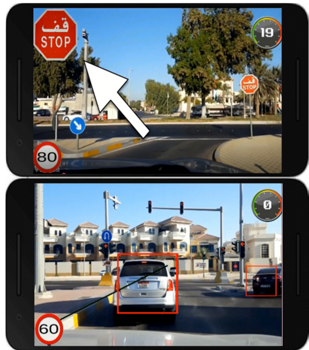
Fig. 9 Drive mode screens (sign detection and collision warning).
