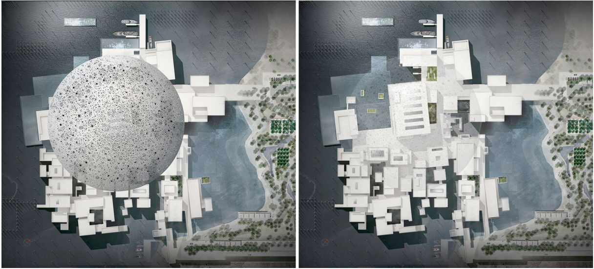
Figure 15. Louvre Abu Dhabi, UAE, 2017, by Ateliers Jean Nouvel, (left) roof plan with the dome; (right) roof plan without the dome, courtesy of TDIC - Architecte Jean Nouvel
