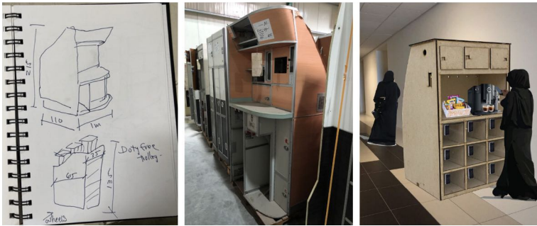
Figure 3 Example of devised process from the survey, measuring, representation and design proposal (Image and photographs by authors)
