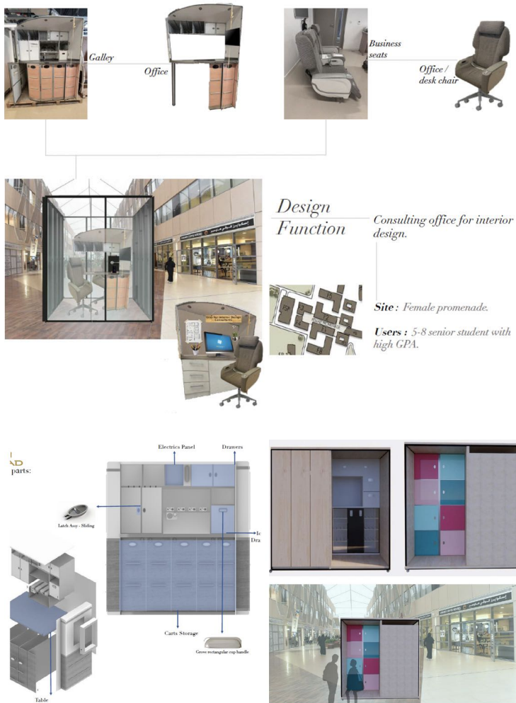
Figure 6 An isolation cabin constructed by the aircraft galley and seat (Image by Gray Group students: Ashia Almansoori, Ayesha Alhammami, Mahra Albloushi, Nora Alnahdi, Mouza Almheiri)
