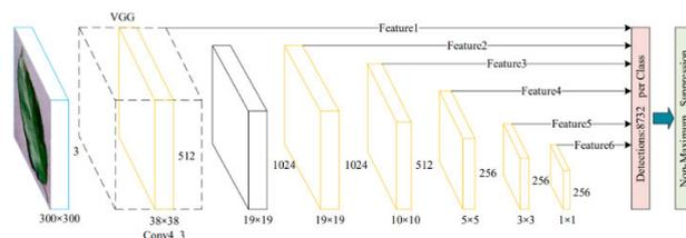
FIGURE 2. SSD network structure [20].
