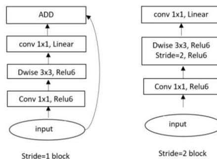
FIGURE 3. MobileNet v2 architecture [23].
