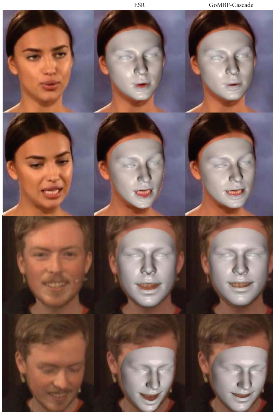
FIGURE 4: 3D facial tracking where GoMBF-cascade tracks faces (globally optimized modular boosted ferns) better than the explicit shape regression (ESR) model [20].
