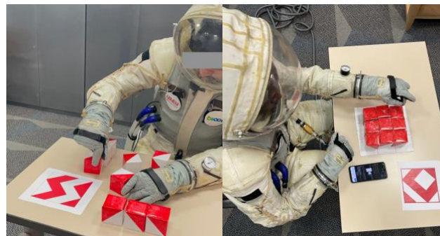
Fig. 2. Two participants undertake their respective Koh Block tests. Left: test is mid journey, sound transparency OFF. Right: start of the test. Note the smartphone placed on the table used to relay ambient sound to the participant (sound transparency ON).
