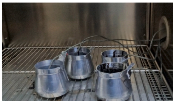
Fig. 1. Temperature regulation test of bitumen and modified bitumen.
